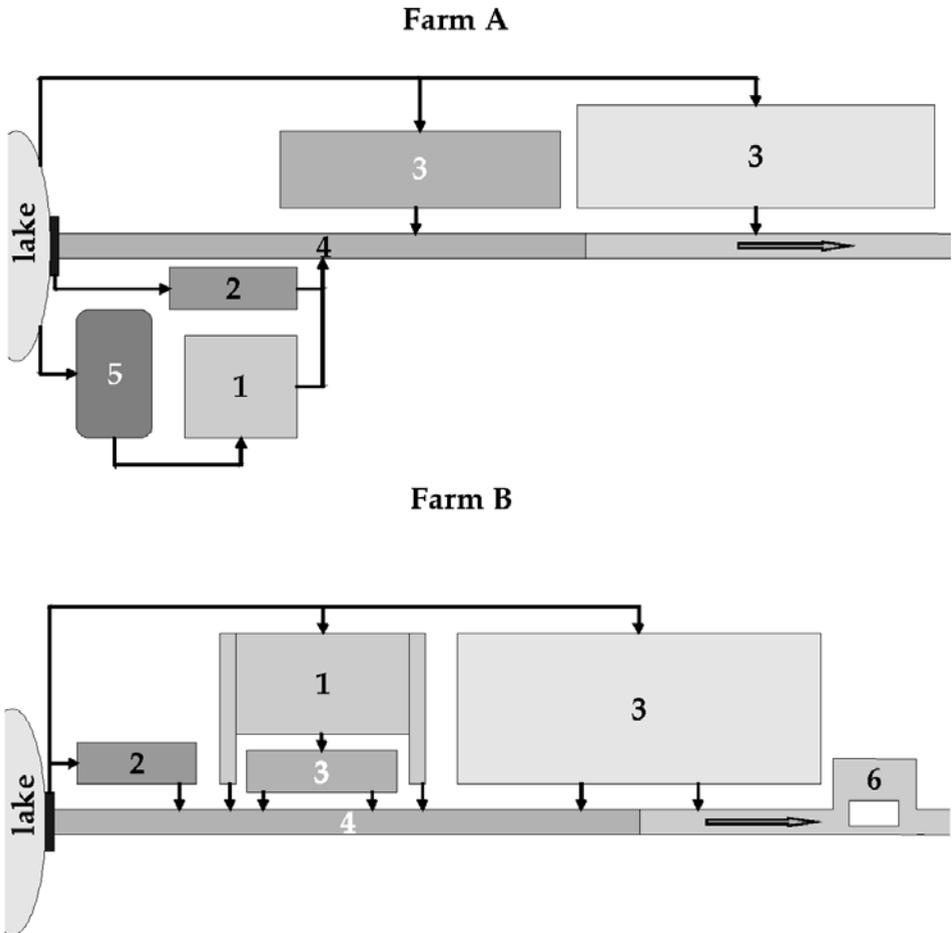
Fig. 2. Technological scheme of trout farms A and B: 1 – grow-out trout ponds, 2 – hatchery, 3 – earth grow-out ponds, 4 – production barriers in the river, 5 – water mixing zone, 6 – settling pond.
