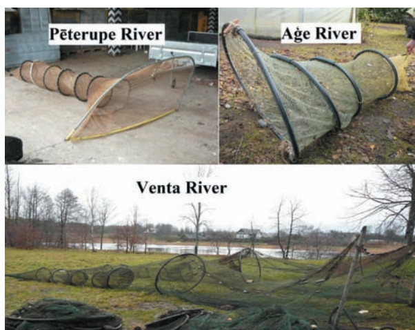
Figure 2. Design of the “regular” lamprey fyke net in some rivers – Pēterupe River (fishing ground No. 6); Aģe River (fishing ground No. 4); Venta River (fishing grounds Nos. 14a and 14b).
