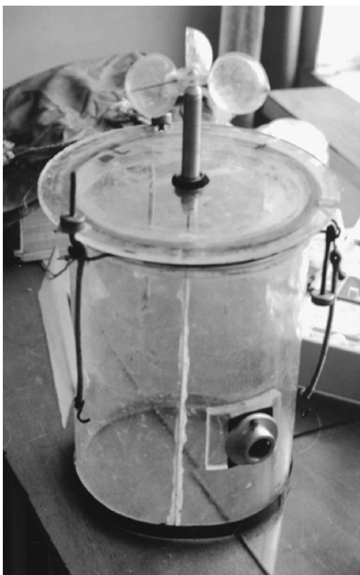
Phot. 1. Respirometer for benthos and periphyton respiration measurements "in situ".
