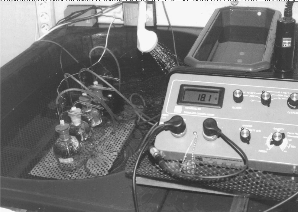
Phot. 1. Botle respirometers used in the experiment
