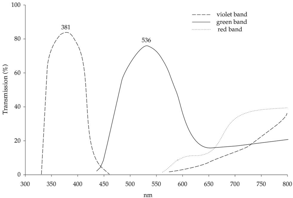
Fig. 2. Spectral ranges of the light transmitted through the filters used in the experiment. All the glass filters transmit some amount of long waves.
